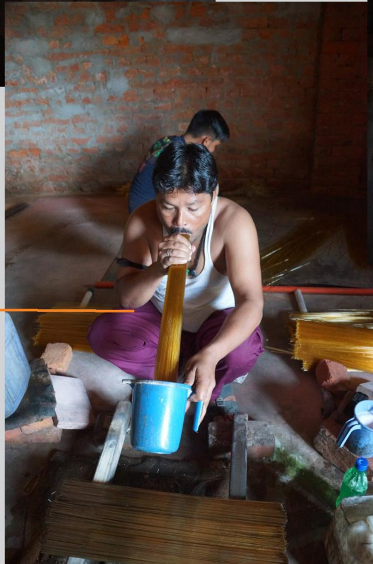
An old traditional method for colouring clear hollow tubes using suction is demonstrated here.
