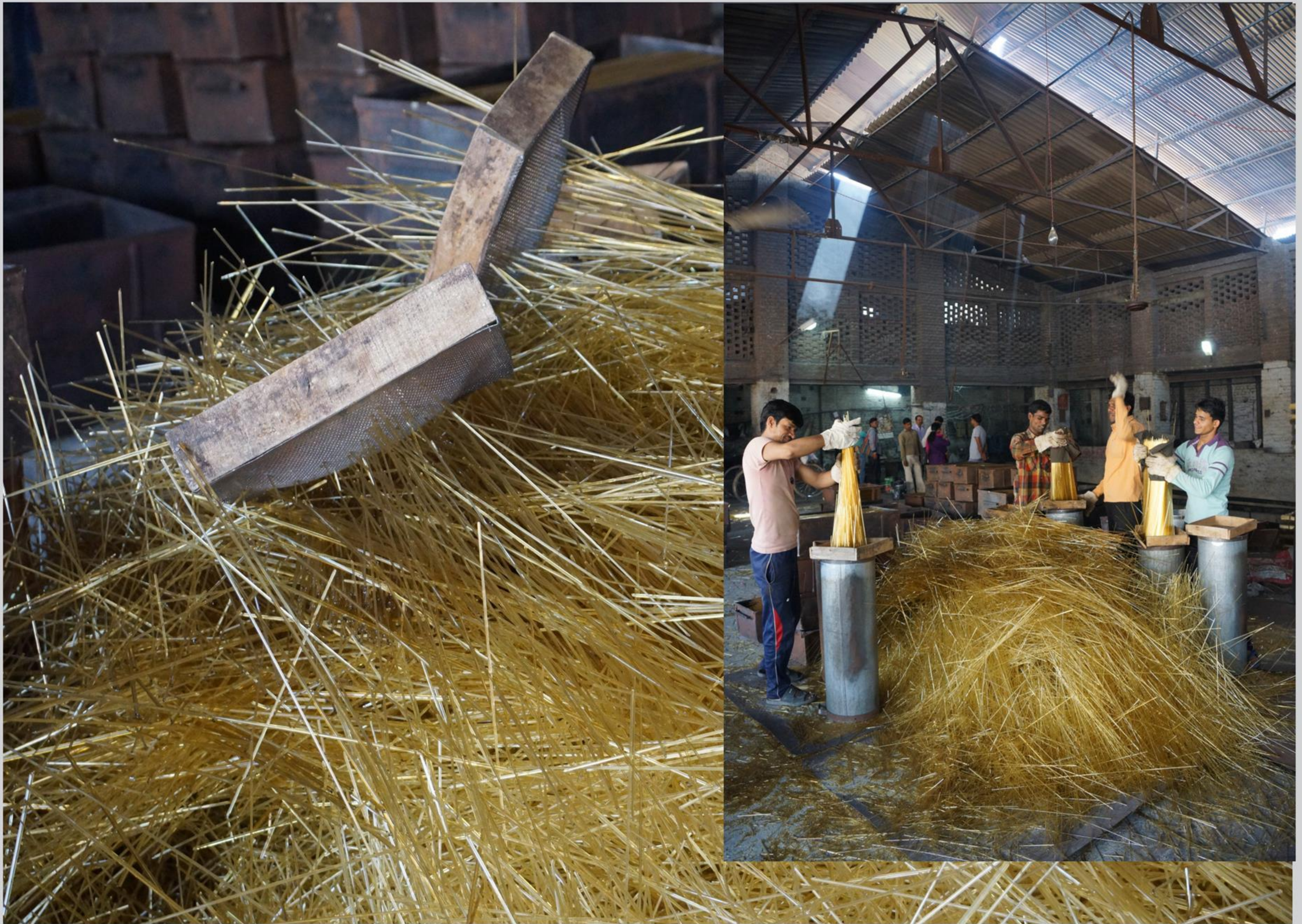
Glass tubes are put through a sieve for measuring width. Those which are too thick become stuck in the sieve and are rejected.
